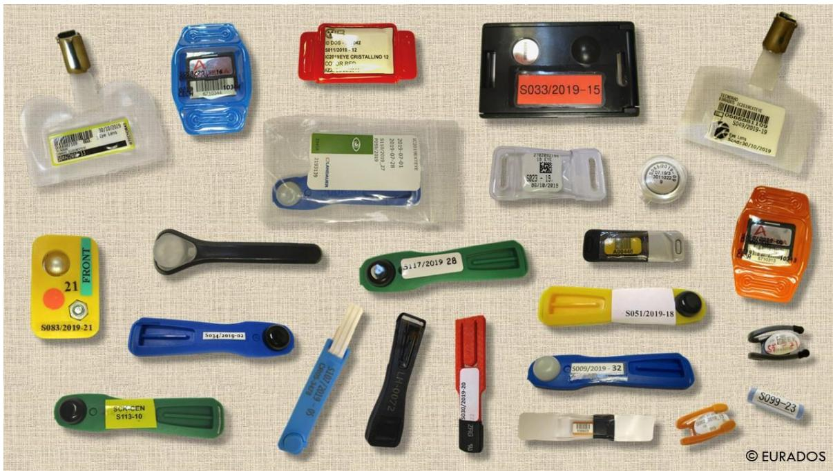
Figure 3: Representative selection of eye lens dosimeters
