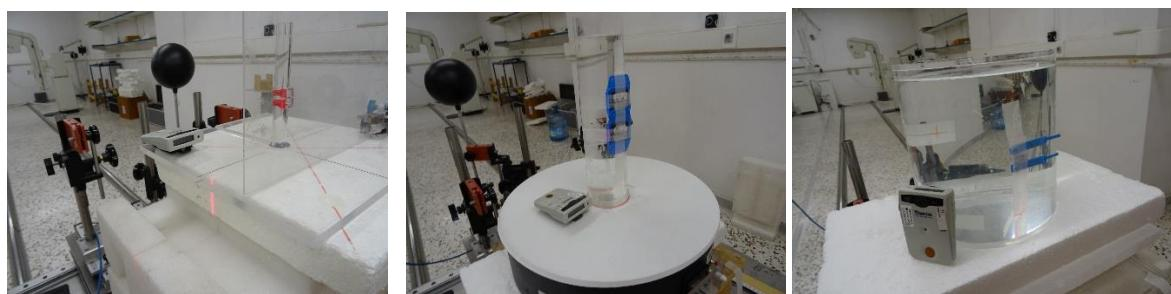
Figure 6: Finger, wrist and head phantoms used by GAEC for photon irradiations
