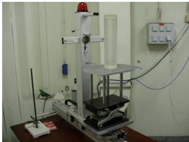
Figure 7: Beta irradiator (ISOTRACK – BSS2) used in this intercomparison
