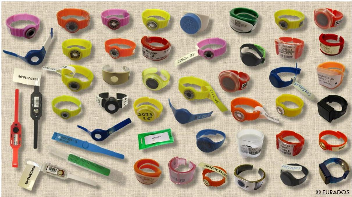
Figure 1: Representative selection of finger ring doseometers
