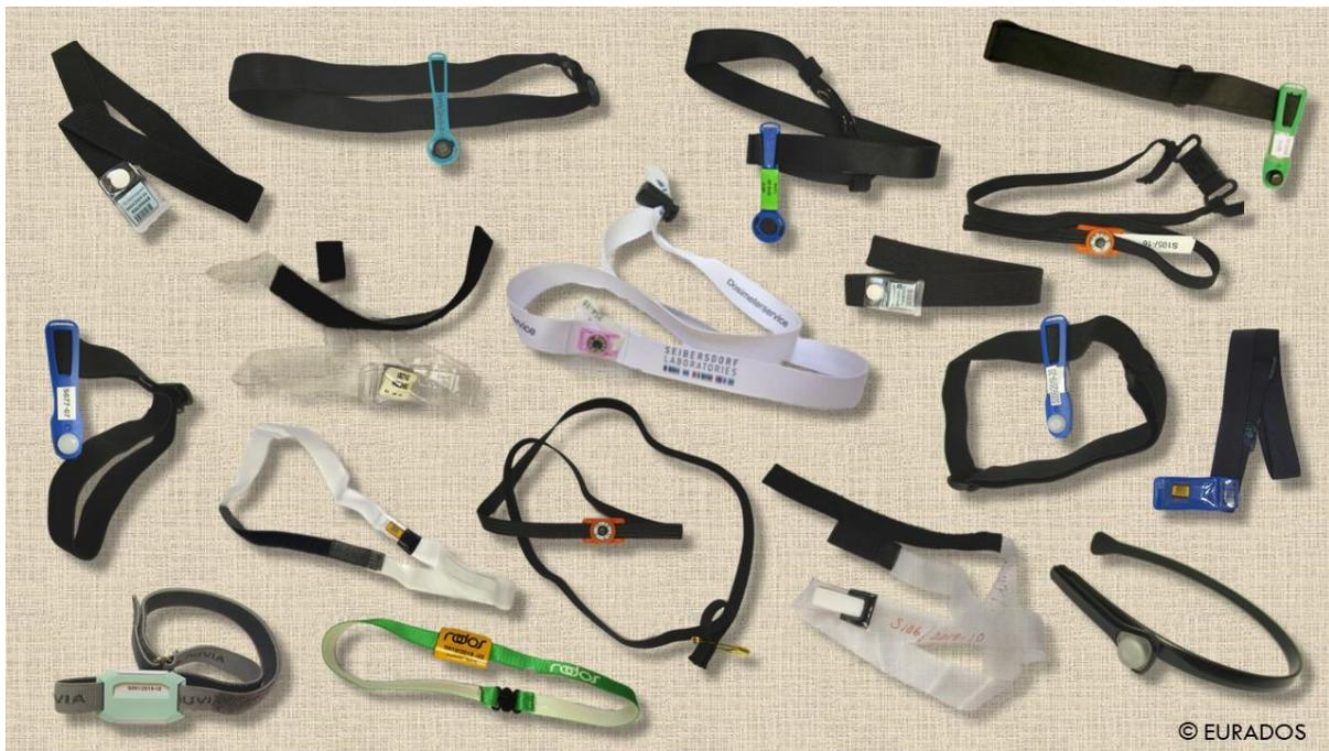
Figure 4: Representative selection of eye lens dosimeters with headbands
