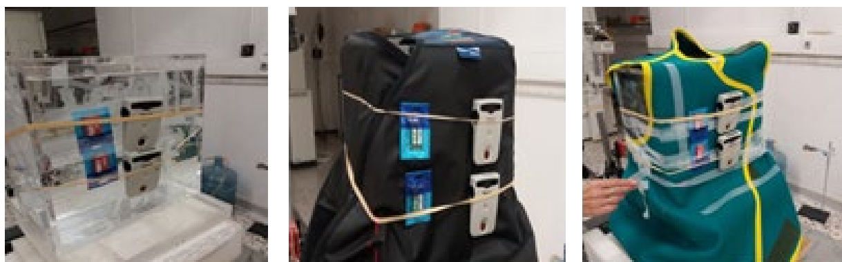
Figure 8: Irradiation set-up using the passive and active detectors on ISO slab phantom (left), with lead apron (centre) and with lead-free apron (right).
