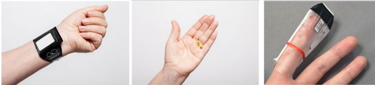
Figure 13: Extremity dosimeters available models. Wrist (left) and ring (centre) dosimeters (source: Spanish National Dosimetry Centre) and finger stall (source: www.ukhsa-protectionservices.org.uk )
