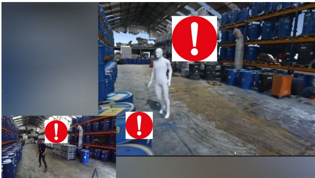
Figure 9.8: View of the camera tracking a worker and the corresponding digital twin reconstruction of the scene.
