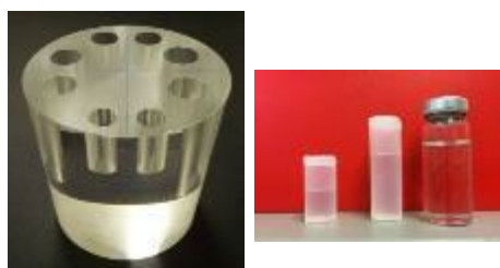
Fig. 4.2: Cathymara thyroid phantom, simulating contamination of ^{131}\text{I} in the thyroid of an adult and 10 years and 5 years-old children, fabricated at SCK-CEN (Belgium).
