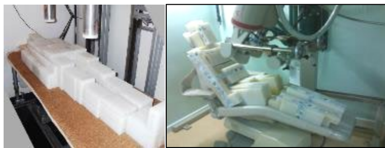
Fig. 4.4: EIVIC brick phantom simulating internal contamination of gamma emitters in total body in an adult individual.
