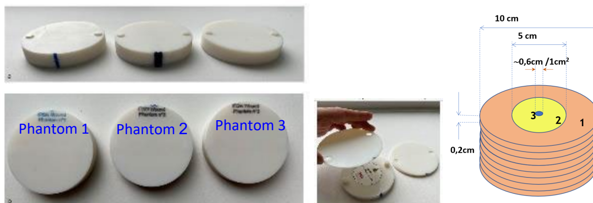
Fig. 4.6: IRSN Wound Phantoms simulating a puncture wound
