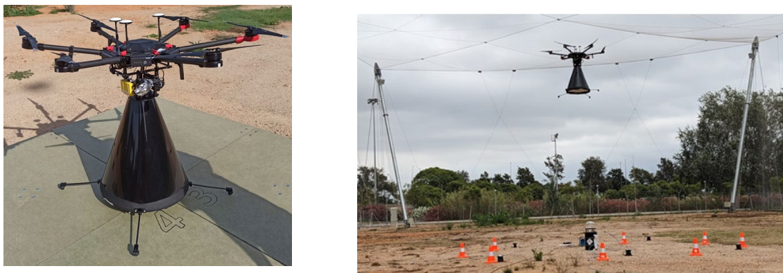
Fig. 6.12: Left: Radioluminescence detection system integrated with the DJI Matrice 600 Pro and ready to fly. Right: Flight performed with the system at the Drone Research Laboratory (DroneLab) of the Technical University of Catalonia (UPC)
