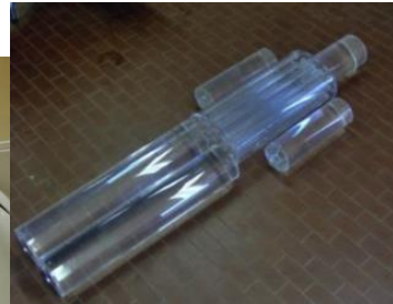
Pipes with TL/RPL/OSL dosimeters
