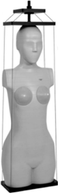
CIRS ATOM female phantom (Model number 702-D).
